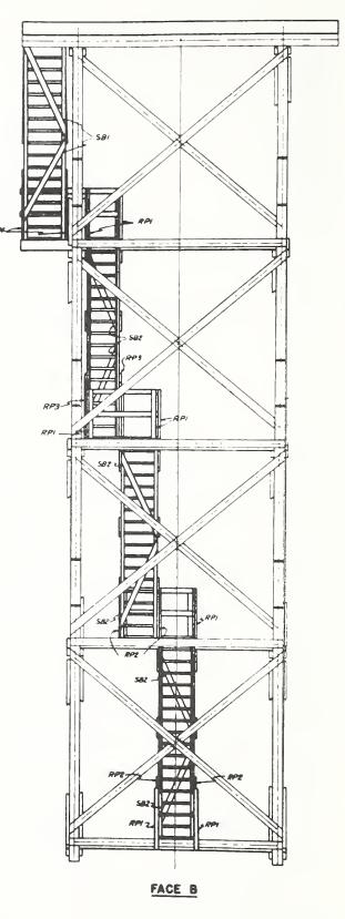
Figure 63. This plan shows the stair layout for the standard timber lookout tower, CT-2 series. It was drawn in 1938 and is 53 feet tall. The plans call for 8 by 8 inch timber for the main posts and 3 by 6 inch timber for diagonals.
